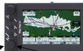
The action always starts by **pressing** on push button of the **left/right** knob or **enter** of remote. After sequenced pressings above mentioned items will be listed on vario display **lower row**. Adjustment is made by **rotary switch** or up/down arrows of the remote. During adjustment process the value is temporary displayed in the lower **right corner** of the display and will disappear automatically after no further commands will be detected.
