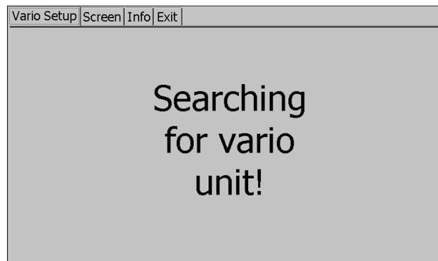
By all versions of MM except KB/V this message shows that vario unit is not connected and therefore no vario settings possible.
