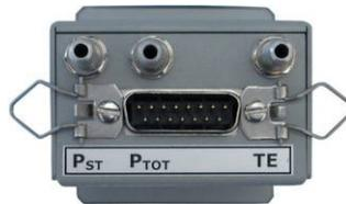
**TE** input should be connected to TE probe, or to statics, if **electronic TE compensation** is intended to be used. Electronic TE compensation should be enabled after using of appropriate setting in navigation program. See also 3.2.2.
